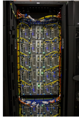
Figure 2.26: A fat tree with a three-level interconnect (left); the leaf switches in a cabinet of the Stampede cluster (right)
