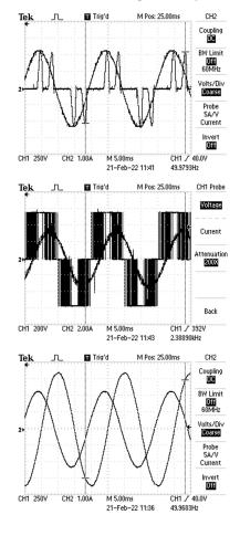
Voltage and current at the input of the speed controller.
