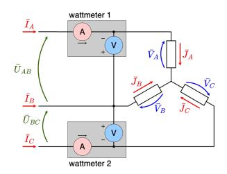
In this configuration, the voltages and currents can be represented on a phasor diagram. Taking  $\bar{U}_{BC}$  as the reference,  $\bar{U}_{AB}$ ,  $\bar{U}_{BC}$ ,  $\bar{J}_A$  and  $\bar{J}_C$  can be expressed as:
