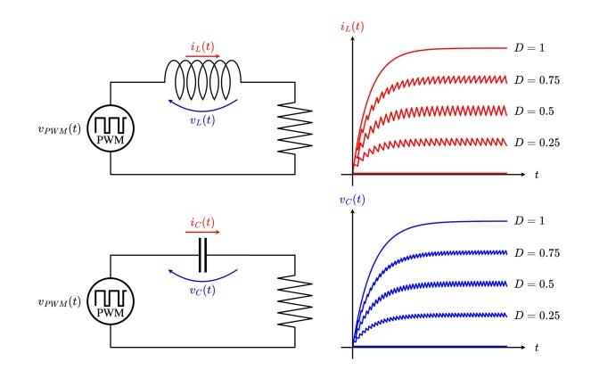
By modifying the duty cycle D, one can control the voltages and currents.
